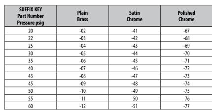
Note: When ordering, specify pressure and finish by adding the two digit suffix after the part number, i.e. 10-407-05: 3/4" FNPT x 3/4" FNPT at 30 psig with plain brass finish.
