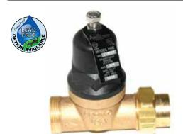
Designed for light duty residential and commercial applications to protect water supplies from excessive pressure. Excellent flow performance at low pressure drop. The dezincification resistant bronze body and dielectric polymer cage provide maximum corrosion resistance. Designed for easy in-line servicing with simple cartridge removal. They meet ASSE 1003 and CSA B356 standards. They are listed with IAPMO and the city of Los Angeles.
